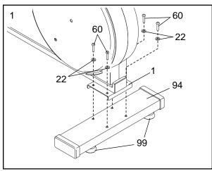
Attach the Front Stabilizer (90) to the Frame (1) with the four M10 x 43mm Button Screws (97) and four M10 Split Washers (22). Make sure that the Front Stabilizer is turned so the Wheels (45) are not touching the floor.
